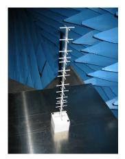
Figure 1: Computer graphics rendering of the best evolved antenna. It is 47 cm high, covers a 6 cm square footprint, and uses 1.587 mm radius wire. There are 15 crossed-elements.
