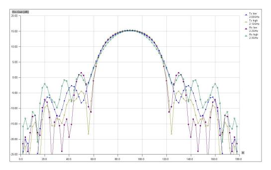
Figure 2: Best antenna gain pattern.  $90^{\circ}$  is on boresight.
